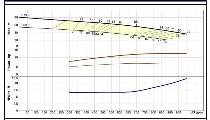
Curve reflects per stage performance for a minimum of 4 stages.
